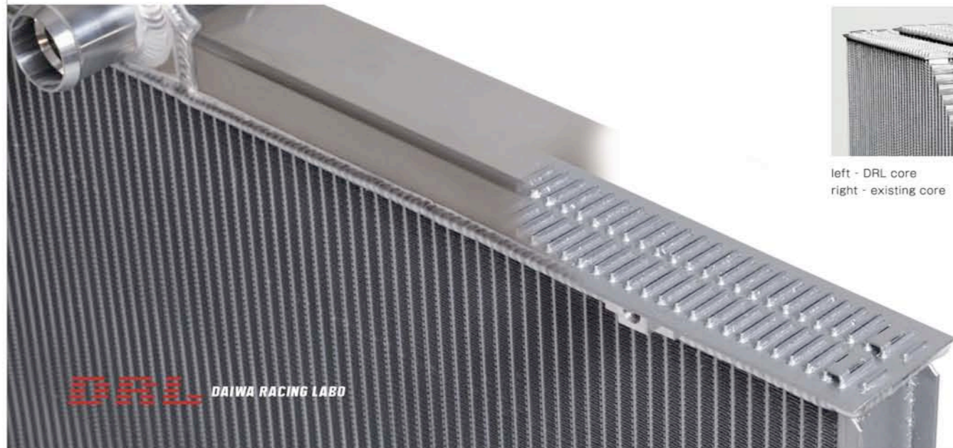
top - DRL designed SQUARE WAVE fin increase the contact area between fin and tube helps the cooling performance and the strength of DRL radiator
